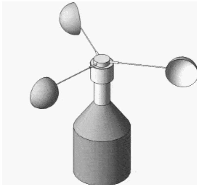
The most widely used Anemometer for **wind-speed measurements** is the revolving-cup electric anemometer. The revolving cups drive an **electric generator**. The output of the generator operates an electric meter that is calibrated in wind speed. **Three-cup anemometers** are currently used as the industry standard for wind resource assessment studies & practice. You may use Ultrasonic Anemometer if you don't want movable parts.
