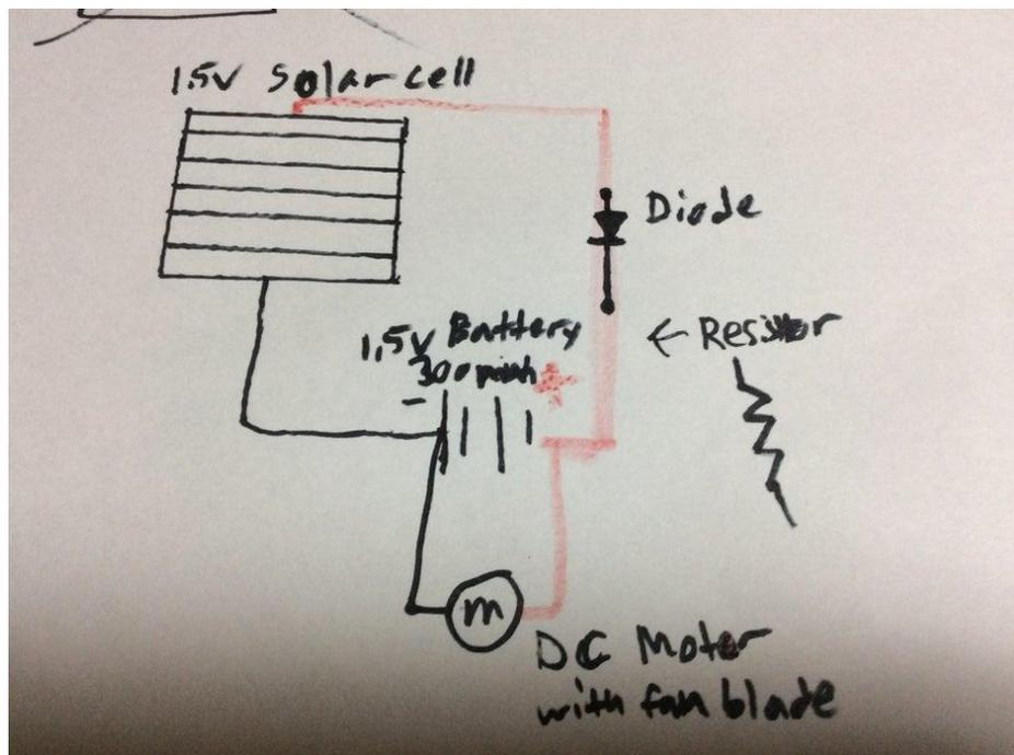
The circuit itself is pretty basic and the diagram shown will show you the layout of the components in the circuit. If you are using different batteries or components to increase the voltage then swap the out with the ones I have used. The resistor amount will be determined by your set up, depending on what type of battery you use or the solar cell you choose.
