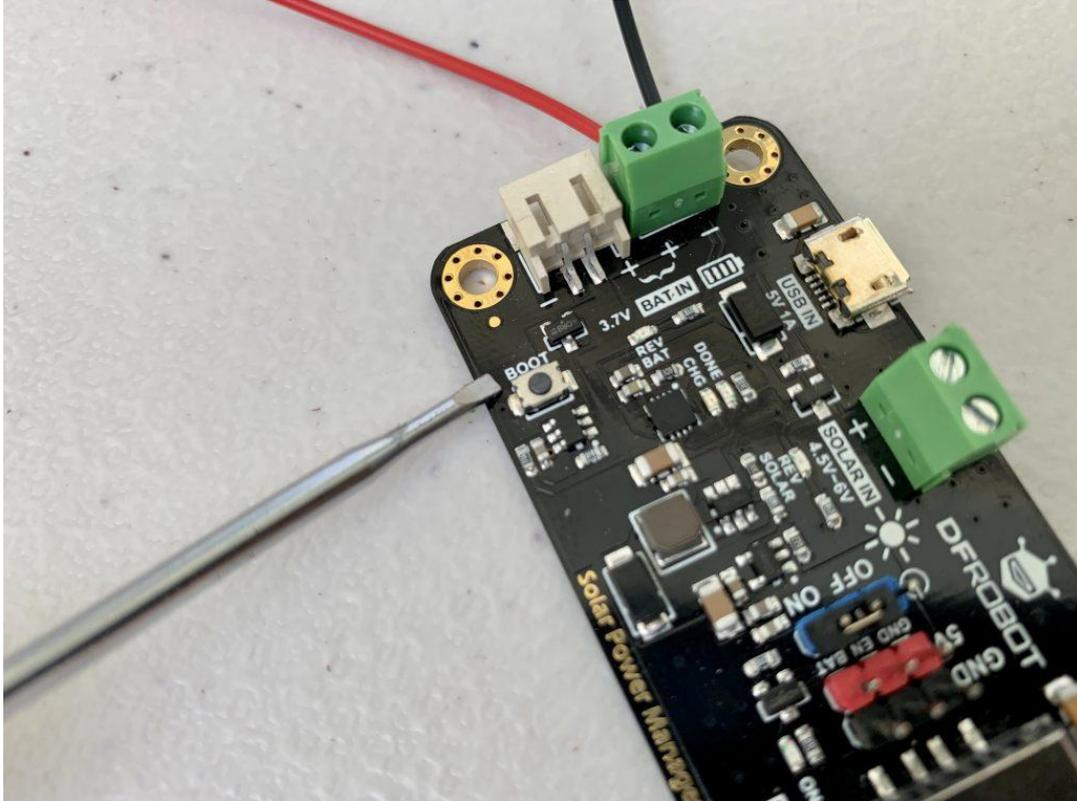
Press the **BOOT** button to turn the board on. Once you do, you should see the ON light turn on.
